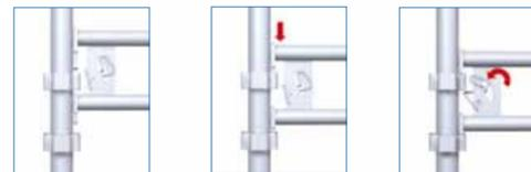
The spring locking catch is primarily designed for manual locking. The catch can be moved easily with the thumb to a distinctly locked or unlocked position. The spring locking catch makes it possible to erect from distance. There is no risk of any moving parts of the construction jamming as a result of painting, blasting and corrosion.
